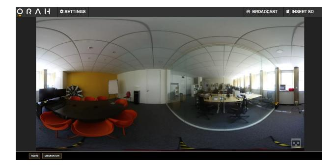
The web control application features a live preview, options to view and change various settings for the stitching box and the Orah 4i camera, as well as controls to start/stop broadcasting live content on the Internet and record to an SD card.
